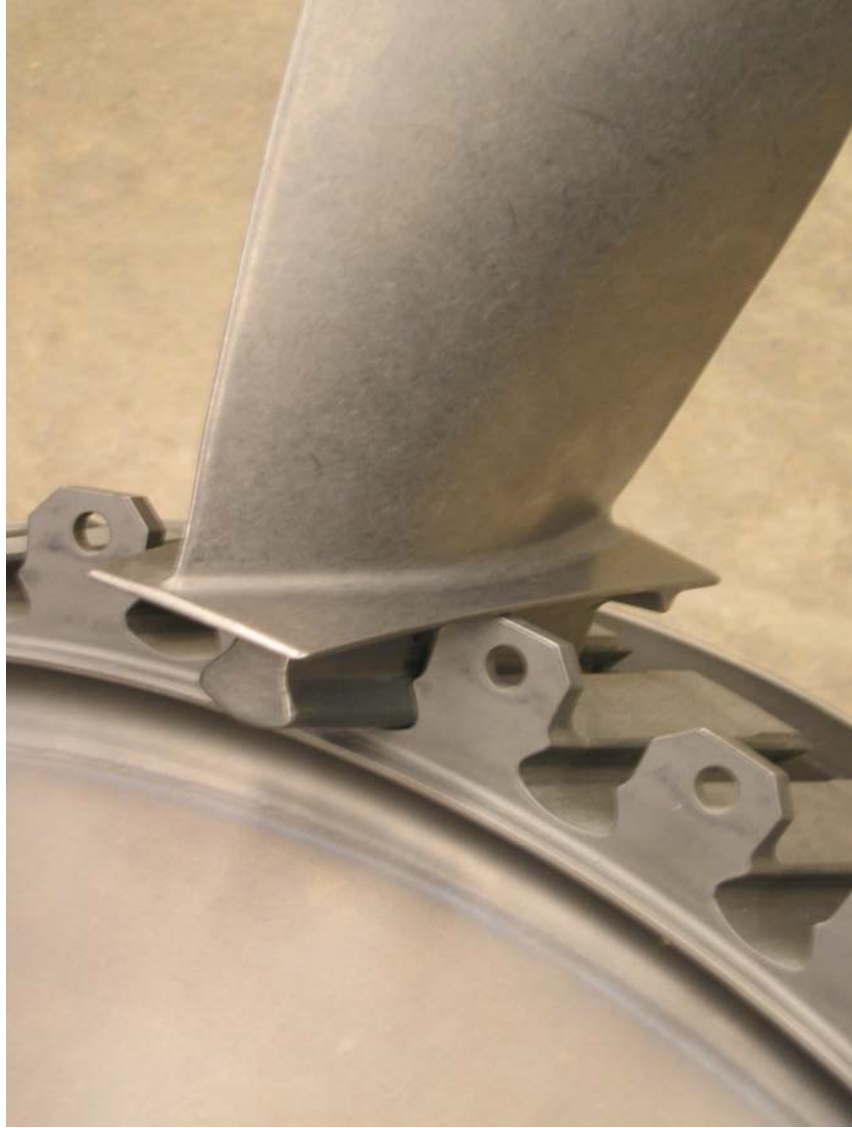
Figure 1. Blade/Disc Dovetail Joint in a Turbine Engine.
